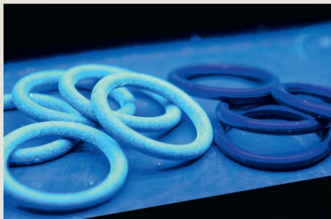
Fig.: Coated seals with ultraviolet indicator (on the left)
